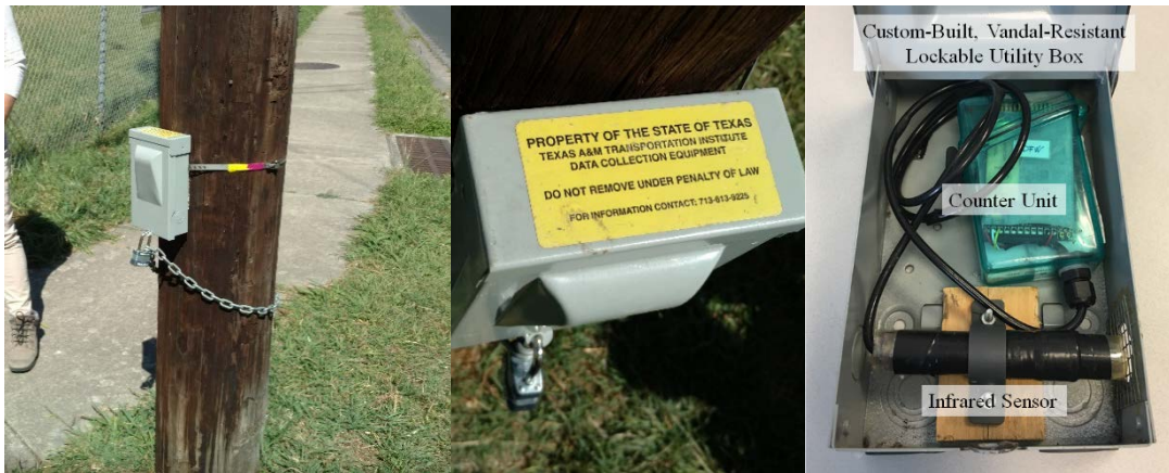
Figure 10. TRAFx Trail Counter Deployed and the Inside of the A/C Disconnect Box.
